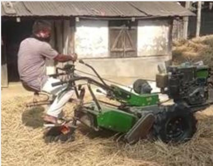
If proper spacing between the paddy is applied during transplanting, then power tillers can be used to till the soil to uproot weeds and other foreign matter. However, the field needs to be dry and firm to carry that out.
