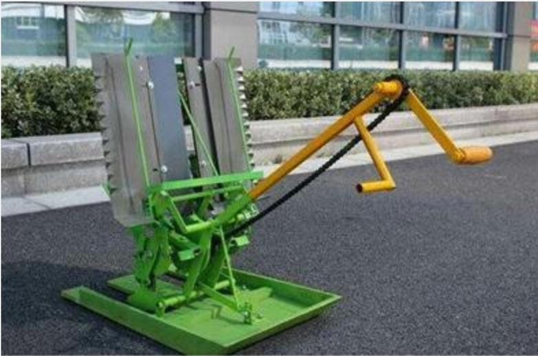
Though the manual transplanters work on the same principle as that of the walk-behind transplanters, they are manually powered and not dependent on fuels like petrol or diesel. Due to its dependence on manual power, these transplanters are limited to planting only 2 rows of paddy at a time. Basic two row transplanters are powered by one hand turning the crankshaft which powers the transplanting mechanism while the other hand pulls the machine along the main field.
