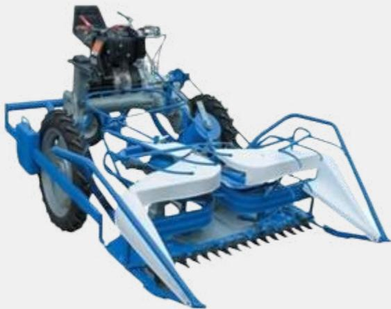
The next level to the reapers are the reaper cum bundler. The machine does all the functions of the reapers. At the end of the cutting cycle, the machine bundles the stalks using specially made strings. Depending on the scale of operations there are both walk behind and ride on variants as well. The reaper binder can also be bought as an independently operated machine as well as a tractor attachment.
