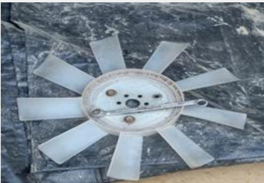
Winnowing of paddy is done using the power tiller. To winnow the gathered grain, a large fan is attached to a rotating shaft of the power tiller and the power tiller is allowed to idle in neutral. Paddy is poured in from the fan which blows away the chaff and light impurities leaving the clean paddy at the bottom below the fan. This is done multiple times until the paddy is clean. In general, it takes about 30 minutes to winnow about 40 kg of paddy.
