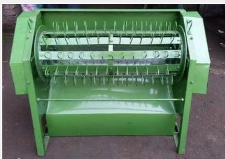
A manually operated paddy thresher is a simple machine used to thresh paddy. Workers press bundles of paddy stalks against the rotating cylindrical cage. The rotating cage knocks off the paddy seeds from the paddy bundles. The rotating cage is powered via a pedal with human power similar to that of a bicycle.
