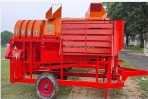
The tractor powered thresher like the name suggests is a thresher capable of threshing and cleaning the paddy. In the first stage the paddy is threshed and in the subsequent stages the paddy is cleaned using blowers. The thresher draws its power from the Power take-off point (PTO) from the tractor. This gives the thresher the flexibility to operate from where the tractor can be driven if the terrain allows for it.
