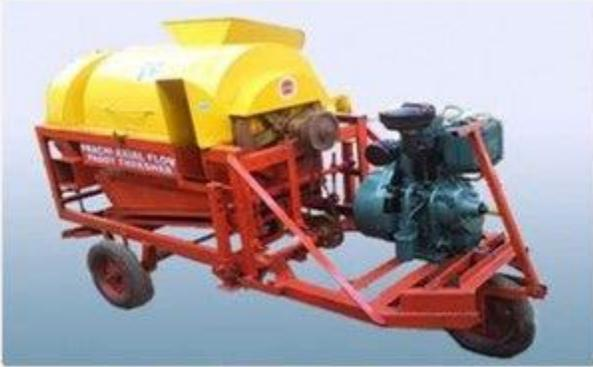
An engine mounted thresher is a small-scale thresher whose mobility is very limited. The rate of threshing when compared to the tractor powered thresher is also lesser as the power input is lower when compared to a tractor.
