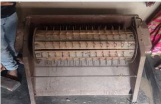
In Jharkhand manually operated paddy thresher was widely used. It is a simple machine used to thresh paddy. Workers press bundles of paddy stalks against the rotating cylindrical cage. The rotating cage knocks off the paddy seeds from the paddy bundles. The rotating cage is powered via a pedal with human power like that of a bicycle. There are also electrically powered versions of the machine as well. Those who do not have this machinery rent it from other farmers.
