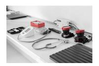
Solar powered battery packs for small portable equipment like Blood Pressure Apparatus, Blood Glucose Monitoring, etc.
