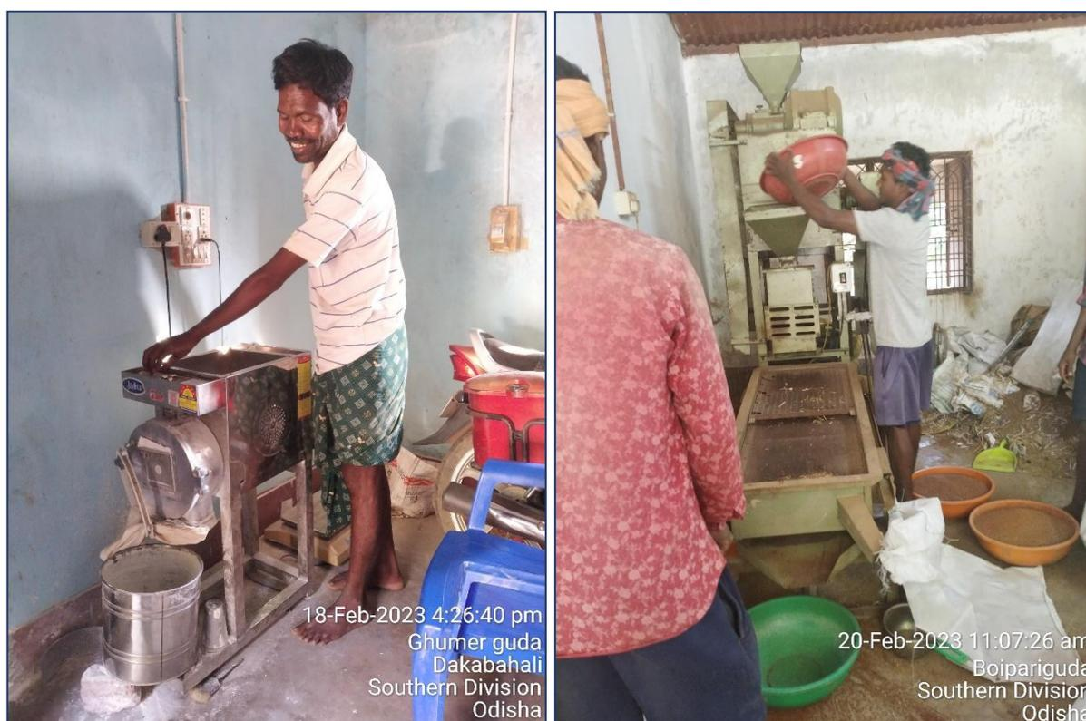
Figure 17. Micro processing Unit for Millets in Bhawanipatna, Destoner and Grader in CYSD Boipariguda
