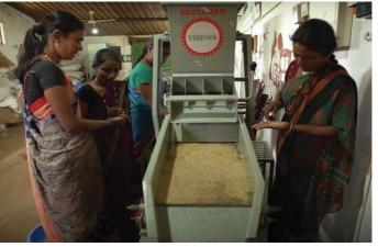
**Proposed Solution** - To enable renewable energy as a resource in post-harvest processing, A 4.5 HP millet processing unit was proposed to the farmer. Training on utilization of machineries was provided post implementation. INR 80,000 was contributed by SHG towards solarisation of Millet Processing Unit
