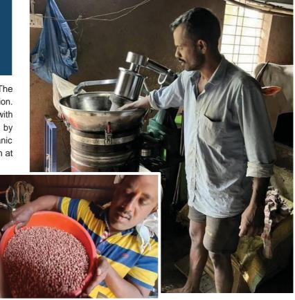
Proposed Solution - To enable renewable energy as a resource in post - harvest processing, A solar powered oil extraction unit was proposed to the farmer. Training on utilization of machineries was provided post implementation. A loan of INR 1,60,000 was extracted from Vijaya Bank for this project.
