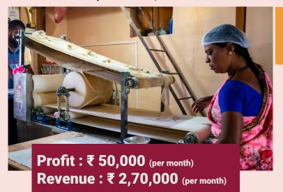
A solar powered conveyor belt roti rolling machine
