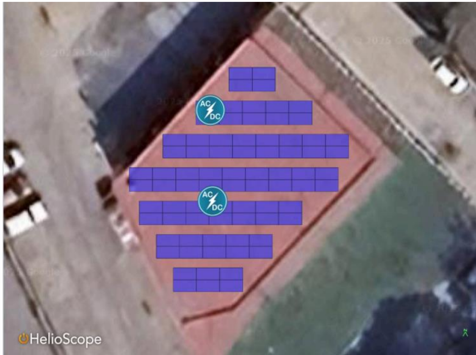
System 3: 45kWp -Fire Station Building– RCC roof – Ballast Type Structure
