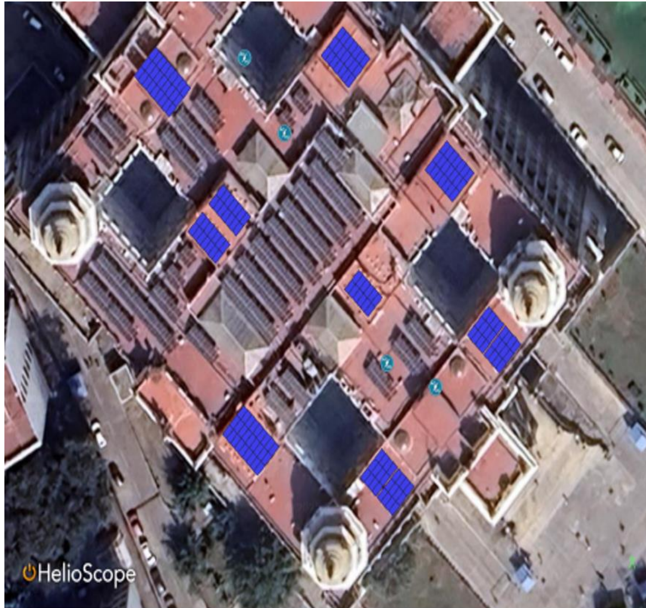
System 2: 102kWp -Vikasa Soudha – RCC roof Structure
